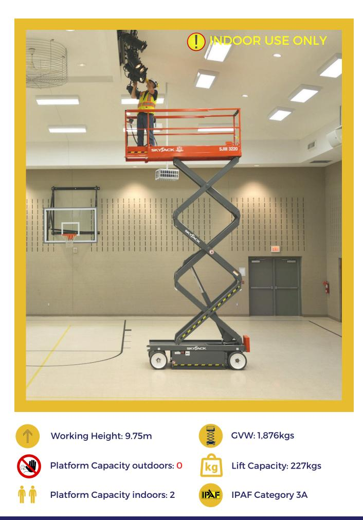
SJIII 3226's are ideal for indoor work where accuracy and precision is critical. 9.75m working height, yet only 0.71m in width. Can pass through a single door, making it an ideal tool for tight spaces. Weighing only 1,876kgs and with non-marking tyres, this narrow electric scissor lift is a front-runner for work on delicate floors.
