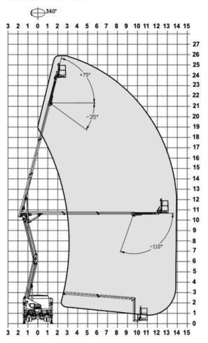
Max Working Height: 26m Max Horizontal Outreach: 14m Max Cage Floor Height: 24m Max Safe Working Load: 230kg Max Persons in Cage: 2 Max GVW: 7500kg DIMENSIONS
