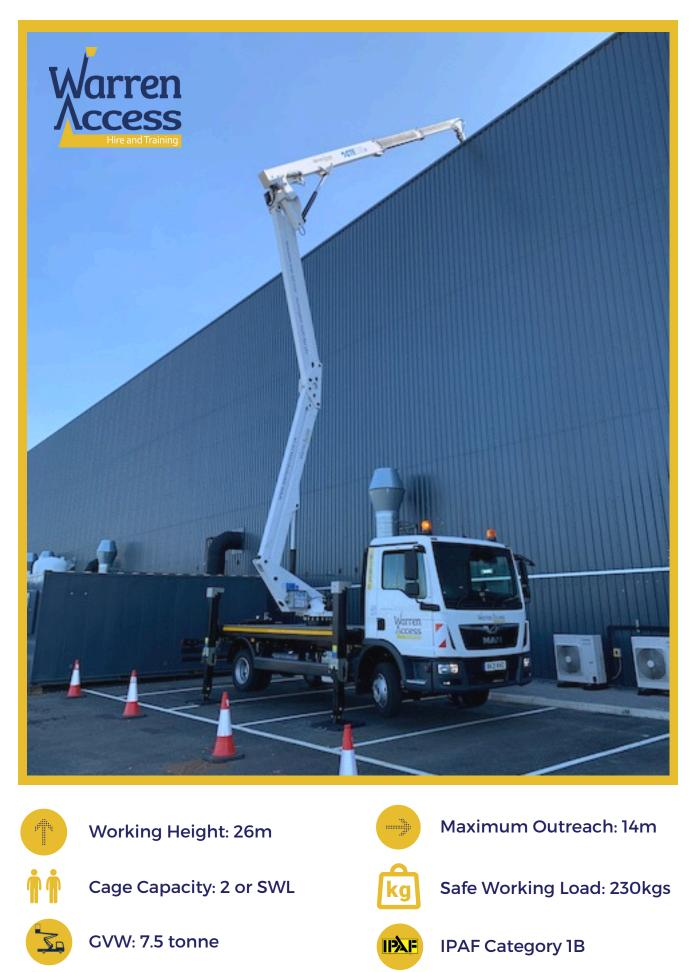
The CTE ZED 26JH has a double pantograph and telescopic boom with two extensions and jib. It has a 26m working height, a horizonal outreach of 14m and very simple controls.
