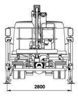
Cage Dimensions: 1.8 x 0.7 x 1.1m Travelling Machine Length: 7.8m Travelling Max Truck Height: 3.3m Travelling Machine Width: 2.8m Working Machine Width: 2.8m Driving Licence Category: C1
