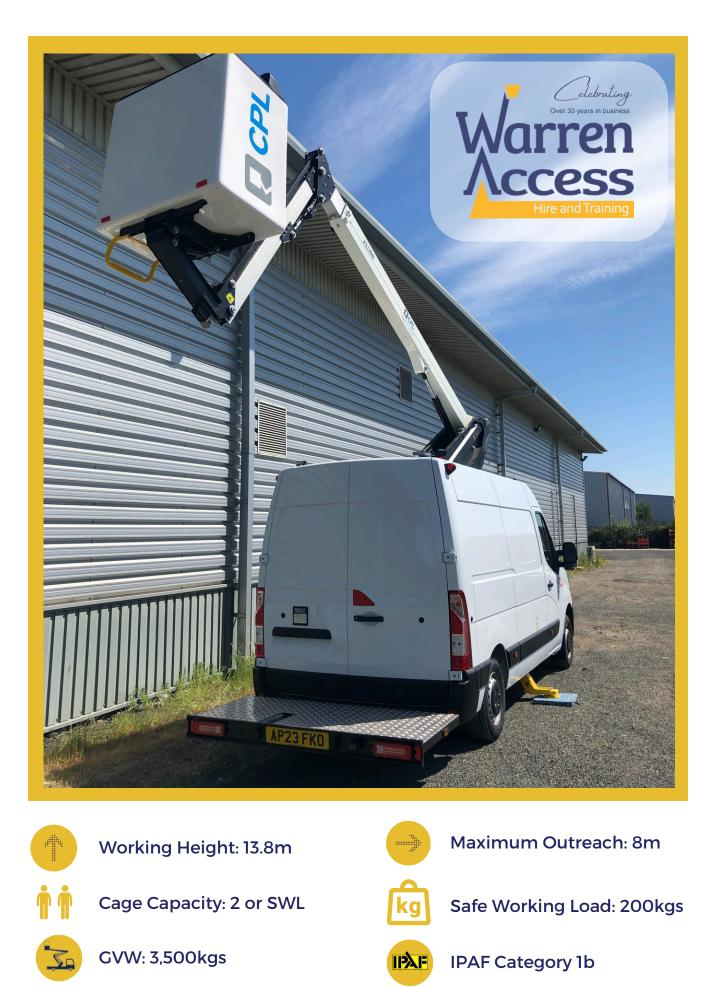
Our CPL K38P van mounted platform has a working height of 13.8m, max horizontal outreach of 8m (when carrying 120kg) and, with an SWL of 200kgs, it can accommodate two people plus tools in the basket. The K38P offers impressive outreach on a 3.5t Renault Master, which can be driven on a standard UK licence.
